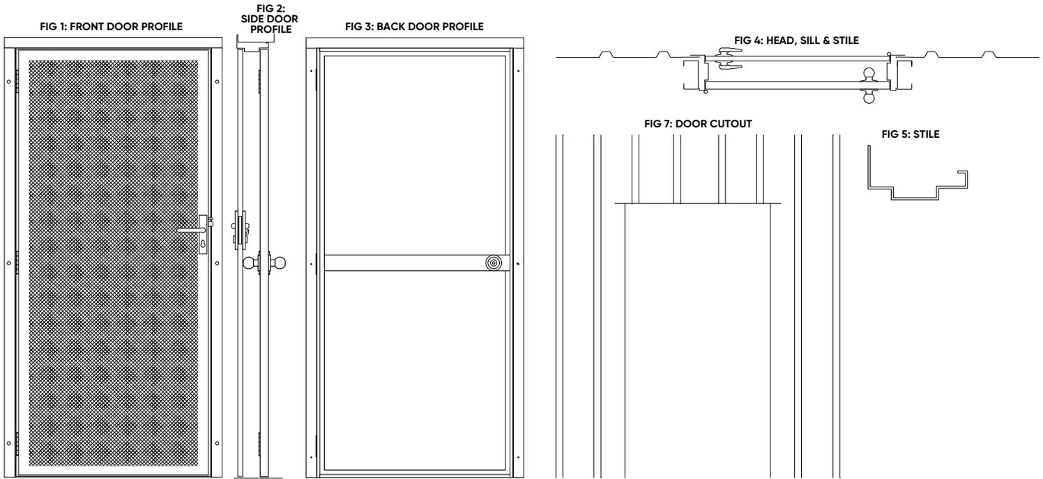
The Sentry® 650.SCR is a combination inward and outward opening, pre-hung door and jamb set.
