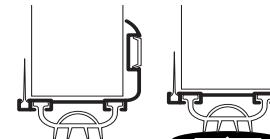
Our 3-sided jamb options include the **Kilargo** bottom door seal, a silver anodised aluminium carrier with grey silicone gasket and cover strip and can be paired with the low-profile **Kilargo** threshold plate to effectively prevent the penetration of cold, smoke, sound, dust, light, insects, and weather, while maintaining all accessibility requirements.
