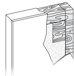
The semi-solid core for the **Sentry® 200 series** consists of medium density polystyrene surrounded by an internal sub-frame made of kiln-dried hoop pine. It includes hardware fixing points for the closer and lock blocks and is fully enclosed on faces and sides with two **Colorbond®** steel sheets, fixed with a two-part polyurethane adhesive.
