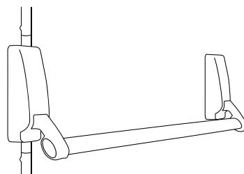
Panic bars are designed to provide building occupants fast and easy egress in an emergency.
